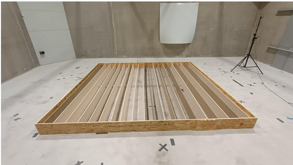
Flat ceiling baffles made from 12 mm PET Fovere felt.
