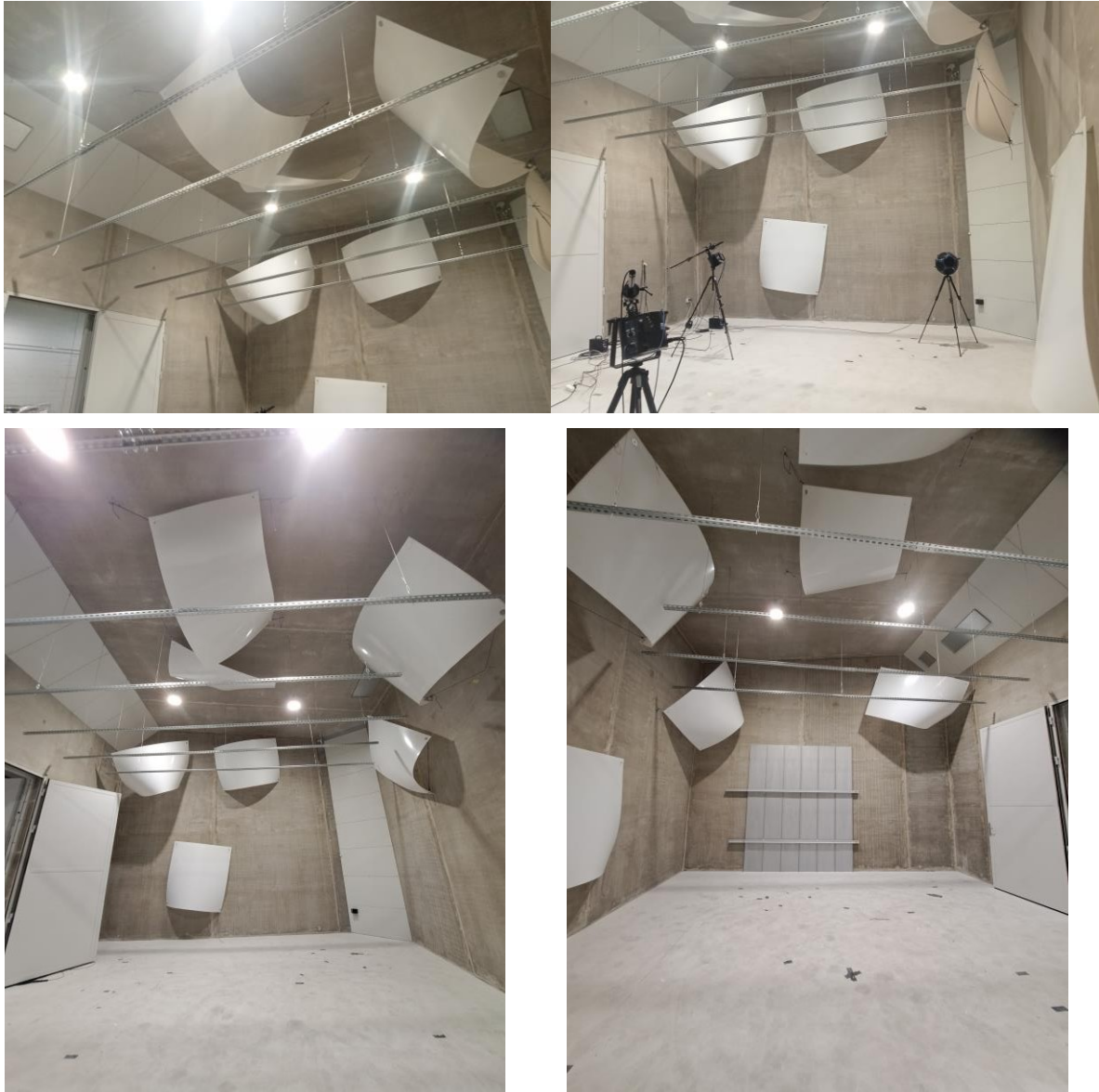
Arrangement of diffusers in the reverberation chamber
